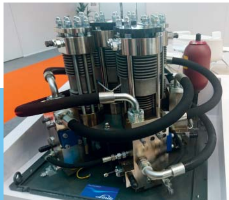
Linde's Ionic container (IC 90)
